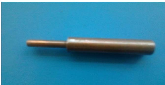
Figure 2: Copper electrode
