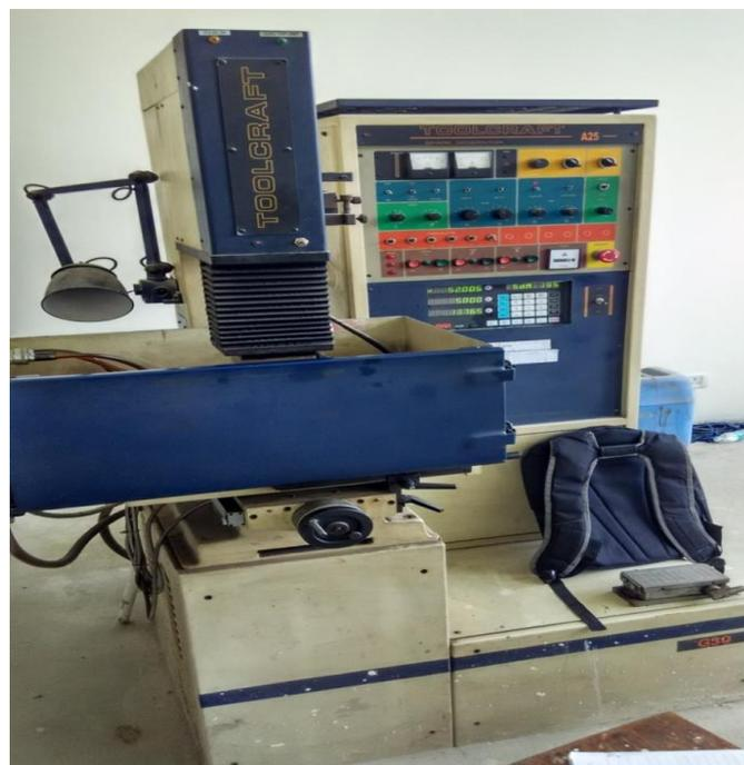
Figure 3 : Electric Discharge Machine, Toolcraft NC machine
